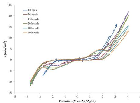
Figure 1. Cyclic voltammograms (CVs) during the treatment of CF composite sample with repetitive scannings in aqueous 0.5 M NaOH solution (scanning rate 200 mV/s).
