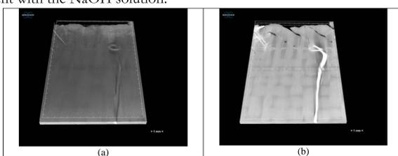
Figure 2. m-CT analysis of the CF composite sample after the electrochemical treatment with aqueous 0.5 M NaOH solution (a) external surface of the composite, (b) internal surface.
