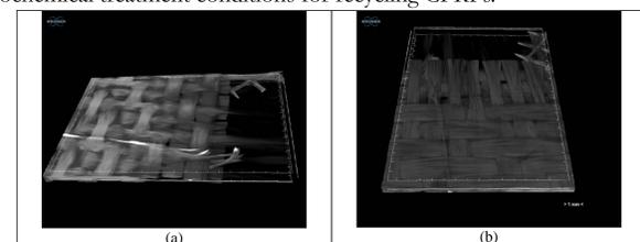
Figure 4. m-CT analysis of the CF composite sample after the electrochemical treatment with concentrated H<sub>2</sub>SO<sub>4</sub> (96%) (a) external surface of the composite, (b) internal surface.
