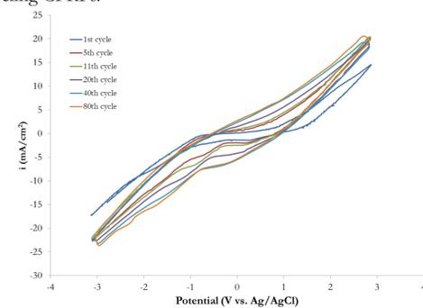
Figure 3. Cyclic voltammograms (CVs) during the treatment of CF composite sample with repetitive scannings in concentrated H<sub>2</sub>SO<sub>4</sub> (96%, scanning rate 100 mV/s).
