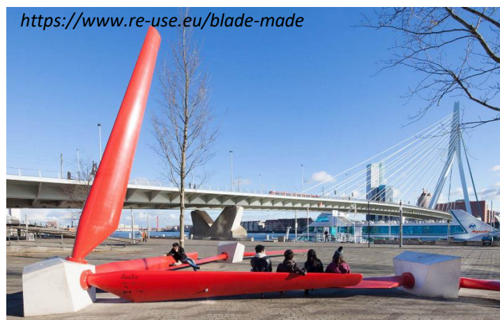
Willemsplein public seating: urban seating using 9 of 6 m WTBs was designed and installed in a Rotterdam square
