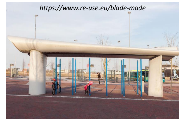
REWIND ALMERE (Bus shelter): convert 30 m blades into pieces of the functional urban architecture
