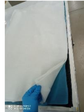
Figure 1. Sequence of the laminate's preparation by vacuum bagging process
