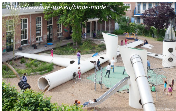
Wikado one-off playground with a similar cost but a smaller ecological footprint using 5 of 30 m blades.
