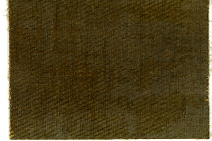
Epoxy/flax fiber prepreg cured by Hot-press
