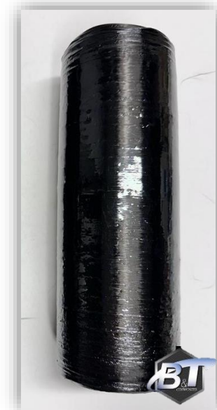
Composite specimen manufactured with Filament Winding
