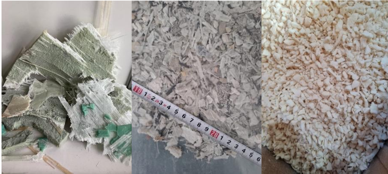
Figure 4 - Shredded and granulated blades - Gees Recycling
