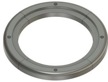
Ø 360 naval window separated in 4 subcomponents
