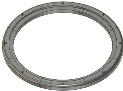
Ø 560 naval window separated in 8 subcomponents
