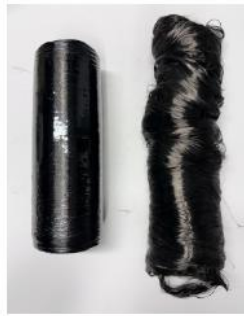
B&T shaft and recovered continous 24K carbon fibre
