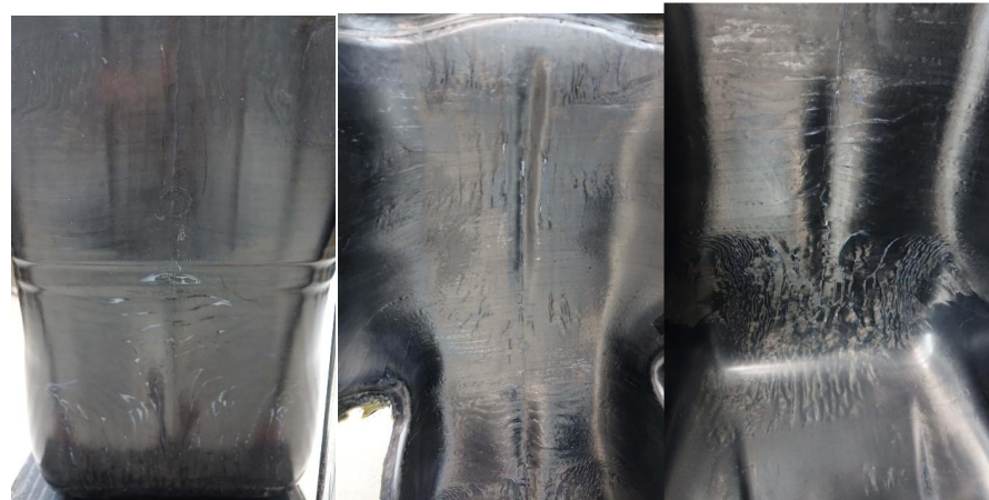
rCF seat upper part and bottom area images showing draping defects and some resin accumulation.
