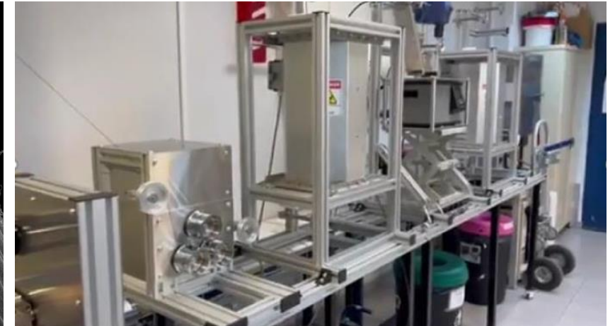
Continuous process for the sizing of CFs to improve handling after recycling process
