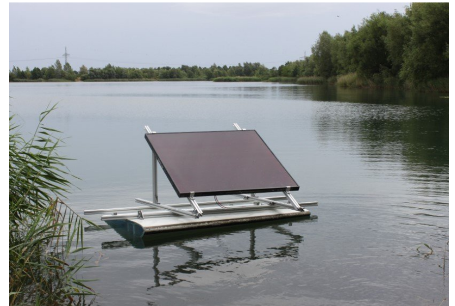
Float test with PV-floating system (HTWK, INEGI)
