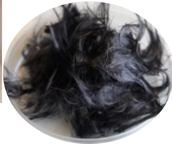
Continuous and short fibres reclaimed by plasma enhanced solvolysis
